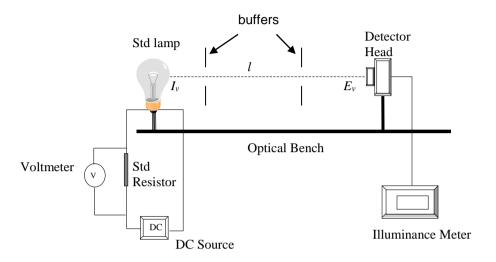
Figure 1: Schematic diagram of the calibration set-up
