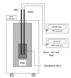
Figure 1:Schematic diagram for PRT calibration
