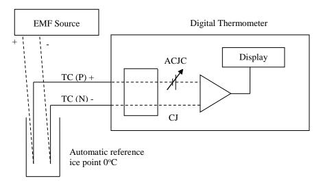
Figure 1: Schematic Diagram for Calibration of Digital Thermometer
