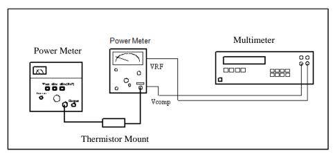
Figure 1: Measurement set-up
