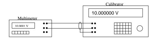
Figure 1 : Connection diagram
