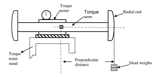
Figure 1 : Set-up of torque tester calibration
