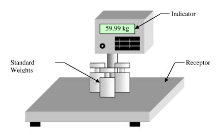
Figure 1: Weighing Machine being calibrated with 60 kg (built up by three 20 kg) standard weights
